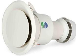
9. The **Univent® h-line™** room outlets are supplied with an inlet tube section which is cut to length to suit the overall wall thickness (from the internal lining visible face through to the face of the external cladding). For thinner overall wall thicknesses, this inlet tube section should not be cut to less than 25 mm from the edge of the plastic weld connecting this inlet tube section to the fan housing.
